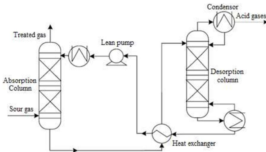
**Figure 1.** Traditional gas purification process based on amine absorption
