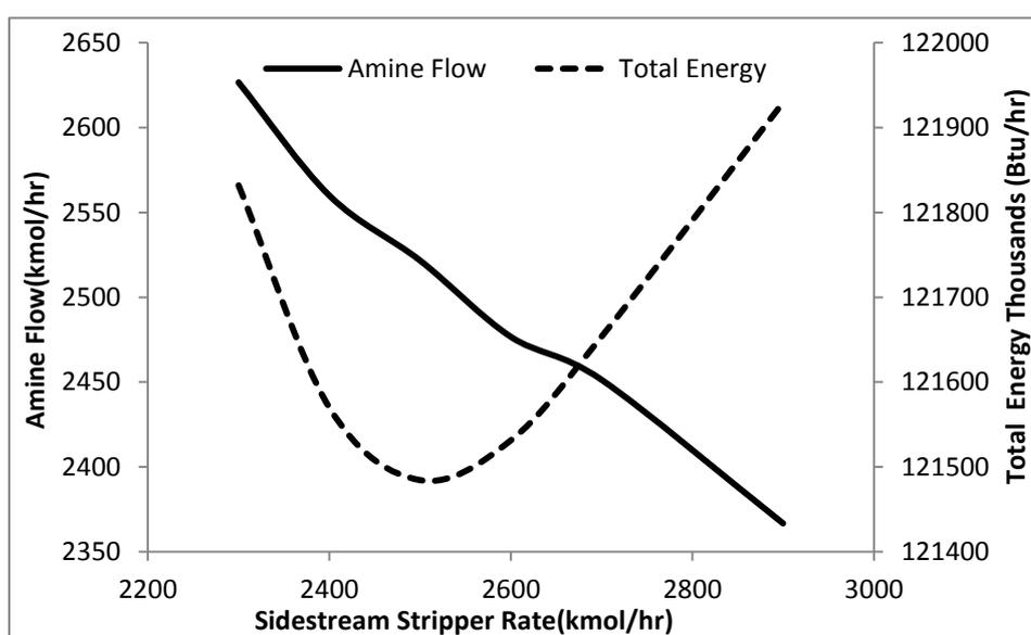
**Figure 2.** Effect of side stream flow rate leaving stage 19 on the amine circulation rate and energy consumption (H<sub>2</sub>S limit: 4 ppm)
