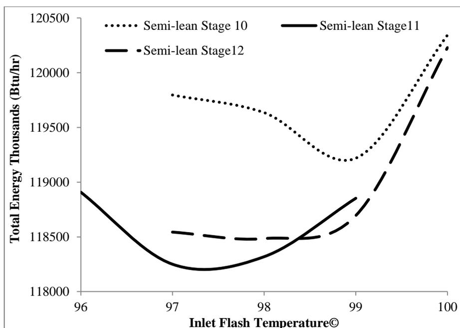
**Figure 4.** Effect of flash unit feed temperature and semi-lean feed stage to absorption column on energy consumption (semi-lean amine stream is entered to absorption column with 28°C)
