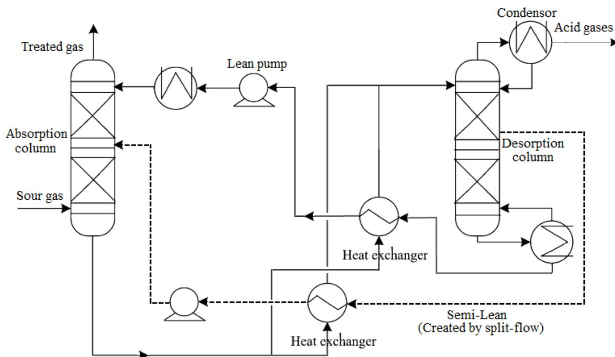
**Figure 3.** Gas purification process (MDEA base) combined to split-flow configuration
