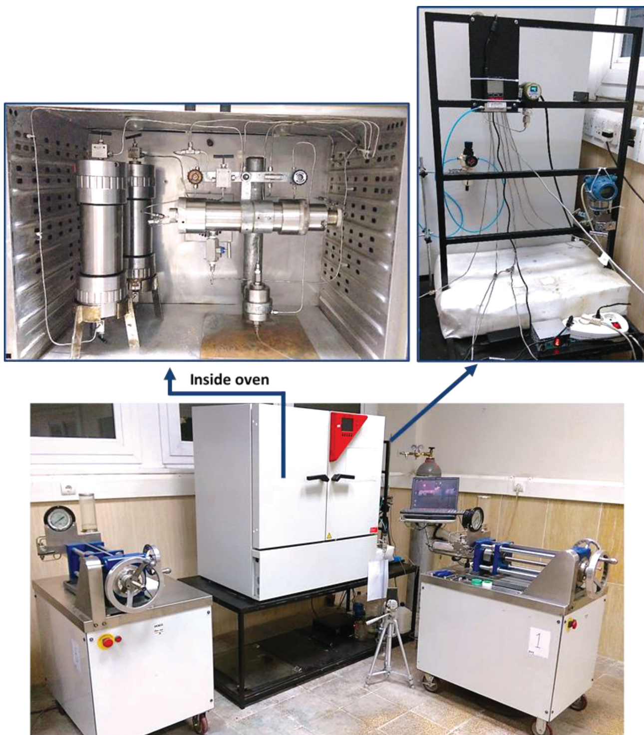
Fig. 1. Experimental set up for core displacement tests and chemical treatment.
